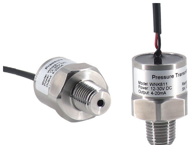
WNK811-B Range: -100KPa~60MPa Accuracy: 0.5% Diffusion Silicon Core
