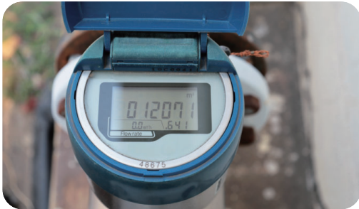
Smart water meter
